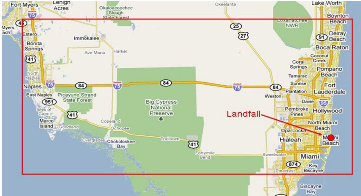
Figure 64 Map Version of Grid for Calculating Hourly Wind Velocities
