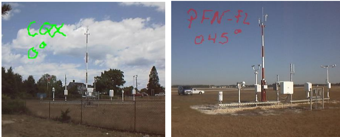
Figure 28. Upstream fetch wind exposure photograph for Chatham, MA (left, looking north), and Panama City, FL (right, looking northeast). After Powell et al. (2004).
