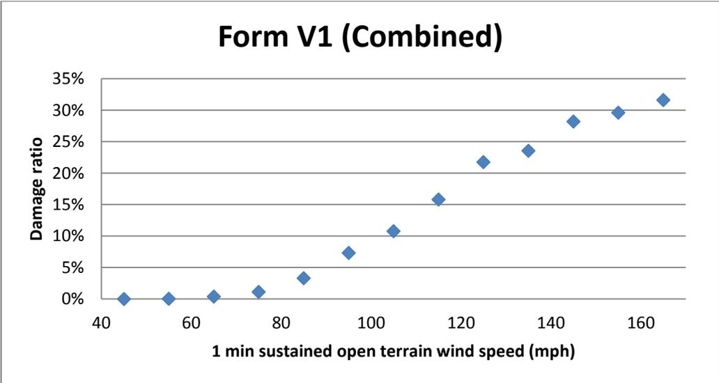
**Figure 110. Structure damage vs. 1 minute sustained wind speed.**
