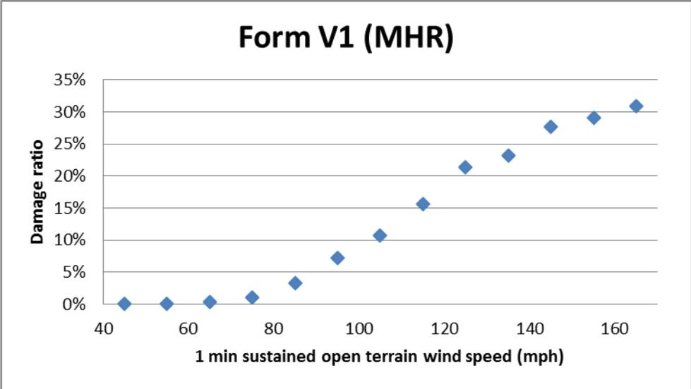
Figure 114. Structure damage vs. 1 minute sustained wind speed.
