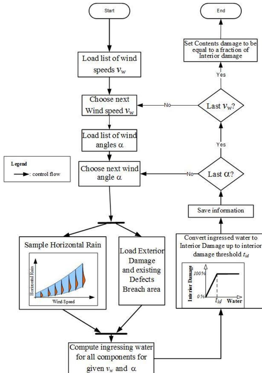
Figure 61. Derivation of contents vulnerabilities for CR.
