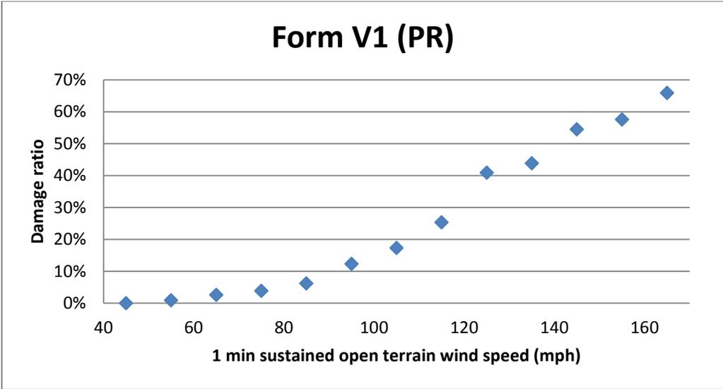
**Figure 112. Structure damage vs. 1 minute sustained wind speed.**
