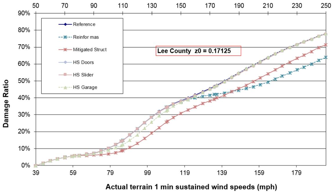
**Vulnerability Curves for Reference Masonry Structure - Mitigation set 3**
