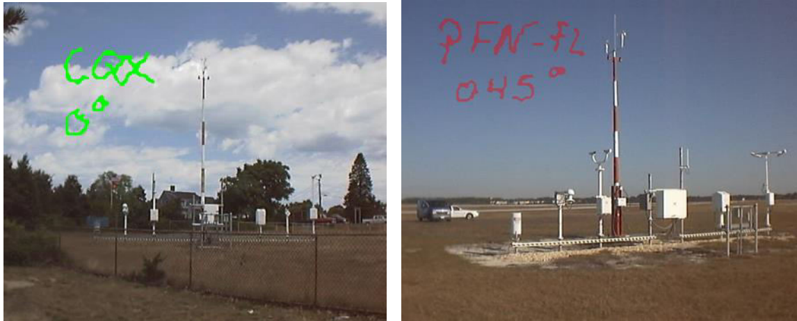
Figure 24. Upstream fetch wind exposure photograph for Chatham, MS (left, looking north), and Panama City, FL (right, looking northeast). After Powell et al. (2004).
