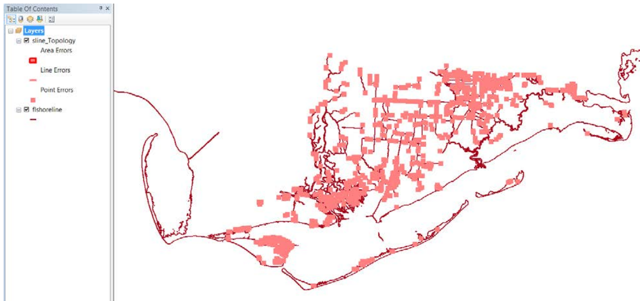
Figure 10. Topologic errors in the shoreline dataset derived from the LiDAR surveys for Franklin County in Florida.
